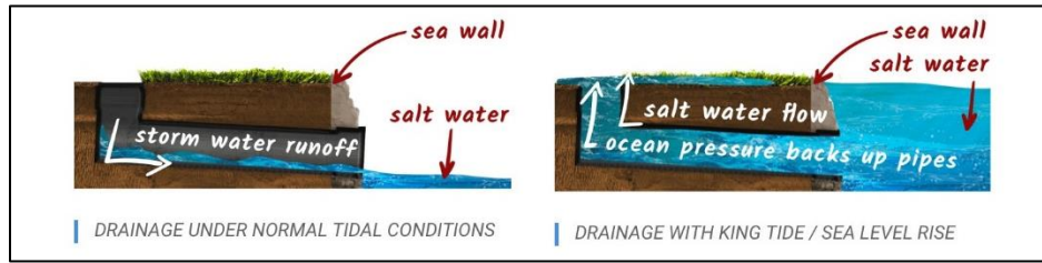
Figure 7, How High-tide Flooding Occurs
