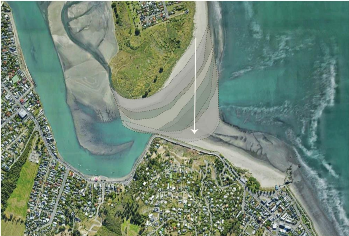
Figure 4. Sand is already accreting onto the tip of the New Brighton sand spit. This diagram illustrates the process by which sand could close the estuary mouth, as more sand is delivered by waves over time. Eventually rising seas could overtake this process, however, and erode the sand gate.
