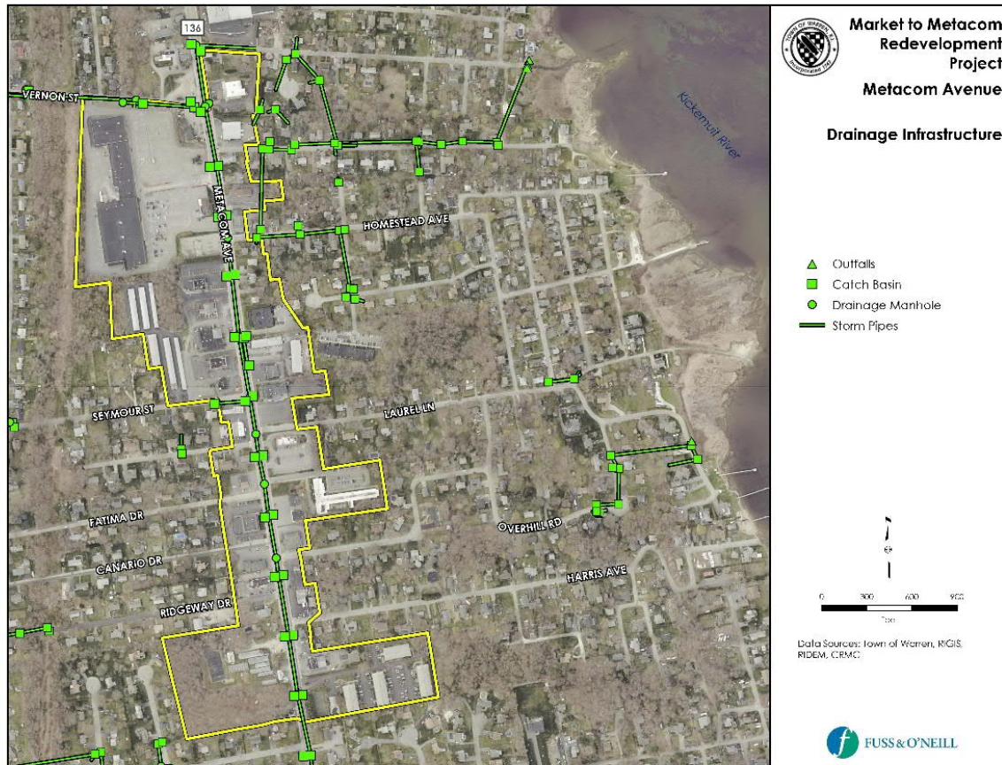
Figure 14. Metacom Avenue Drainage Utilities/Infrastructure
