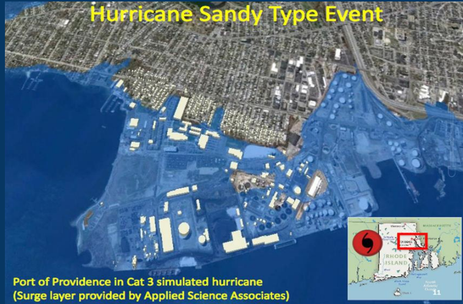
Fig.1. Bathtub inundation of Port of Providence
