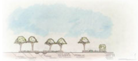
Above: Section view of parking lot entrance with raised walkway and bioswales.
