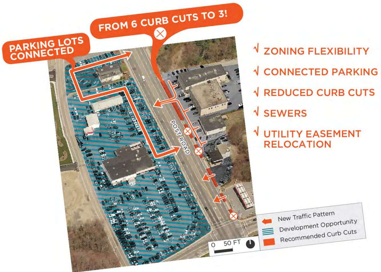
Figure 23. Proposed Post Road improvements to address physical and regulatory barriers to revitalization. Different sets of improvements can help revitalize Post Road including sidewalk improvements, bike lane installation, and curb cuts reductions.
